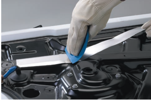
Applied with a 3M™ PA-1 Wiper to the inside of a car door, 3M™ Damping Foil 2552 effectively damps by converting vibration energy to negligible heat that readily dissipates.
