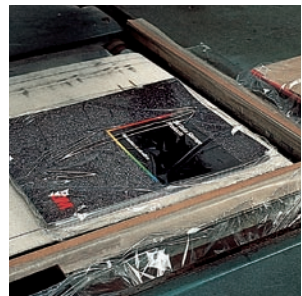
In shrink wrapping operation, 3M™ PTFE Glass Cloth Tape 5451 helps protect the bar underneath where the hot wire seals the plastic film.
